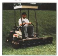
Designed for 700 and 900 Series power units, Grasshopper's 40- and 60-inch AERA-vator™ attachments aerate turf and relieve surface compaction without irrigation, leaving no cores to clean up. Turf is available immediately after treatment. Oscillating. forged-steel tines penetrate and fracture hard, dry soils, encouraging root development and providing a resilient surface for playing fields.
