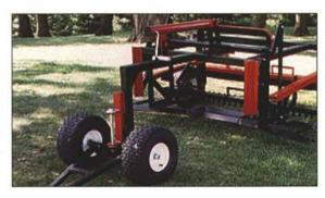
Popular 3 in one machine for professional infield maintenance. This unit has 4 leveling edges, a heavy duty harrow for cutting or aeration, and all weather nylon broom to provide a very attractive finish. This machine can handle from the toughest of conditions, to grooming and finishing the finest of infields.
