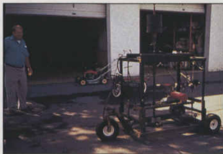
Don Waddington of Penn State stands with the Penn Foot for field traction testing.
