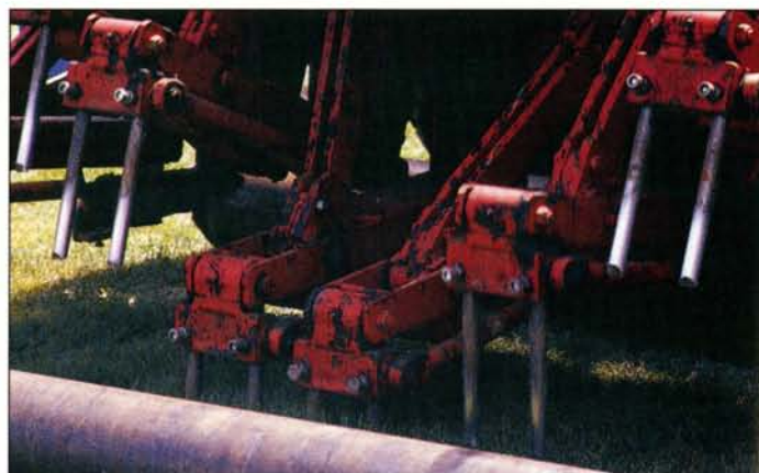
Hollow tines can be used for both conventional and deep aeration.
