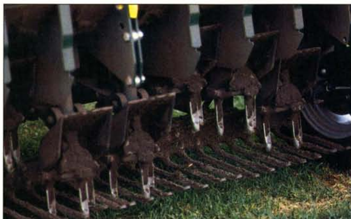
Hollow tines can be used for both conventional and deep aeration.
