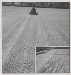
Manufactured of engineered polypropylene fiber in fibrillated form, patented Turfgrids combine with native or select soils to produce a toughened composite athletic surface with increased traction in both saturated and unsaturated conditions.
