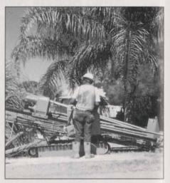
Since multi-use equipment increases productivity and cost return, a good choice may be the L-2 by Line-Ward Corporation. The L-2 is a walk-behind vibratory plow designed for laying cable or irrigation pipe. Its maneuverable in close quarters and its size allows it to get through narrow gates and it has a boring attachment.
