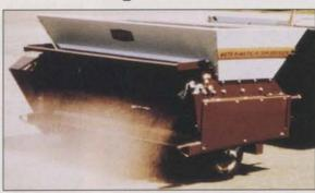
Turfco Mfgs' Mete-R-Matic III topdresser has the new chevron belt for leveling turf and promoting the decomposition of thatch. It is a non-hydraulic ground-driven unit pulled by most tractors and turf trucks. The chevron belt combined with the ground drive revolutionizes topdressers' abilities to uniformly spread material. It has a 5-foot-wide spread and is easily loaded with a front end loader; allowing you to uniformly topdress an athletic field in two hours or less.
