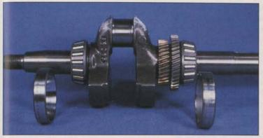
Crankshaft bearings and seals are commoly replaced during overhaul. Excessive vibration that continues after tune-up is often a sign that crankshaft bearings need replacing.
