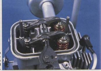
Valves can usually be cleanedup and the valve seats re-ground during overhaul.
