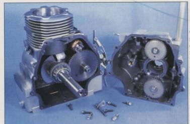
Overhaul generally consists of replacing all those parts that are subject to wear during normal operation, replacing seals and the removal of carbon and sludge deposits in the engine.
