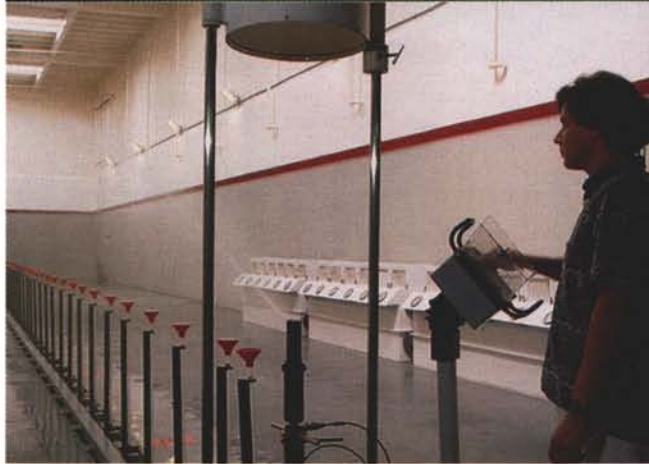
Above: Irrigation at Mile High Stadium in Denver, CO. Left: Single line tests are used by sprinkler manufacturers to help determine uniformity.
