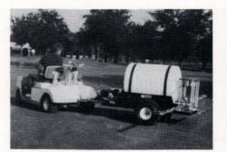
with controlled droplet applicators (CDA)an advanced system of spraying that uses reduced volumes with greater chemical efficiency and optimal control and accuracy. The CDA sprayers deliver droplets in a uniform size, ensuring less drift and less water
