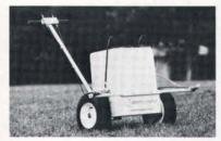
The **Greens Wheelle** is a liquid chemical spreader with a unique grounddriven pumping system. The unit gives the sports turf manager the benefit of a boom-type spreader without the worry of engine maintenance.
