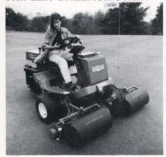
The Bunton line of professional mowers now includes a riding triplex greensmower. The mower is available with either an 18 hp twin-cylinder Onan gasoline engine or a 16.5 hp three-cylinder water-cooled Kubota diesel, both on anti-vibration mounts. The Onan has an aluminum block with cast iron sleeves. The drive is a true hydrostatic, closed-circuit which requires fewer valve banks and hydraulic pumps than other systems for lower maintenance.
