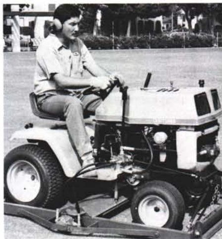
The Haley Planer is a verticutter centered on a six-foot-long frame built for bowling greens.
