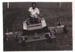
inches wide with rear discharge and can be raised or lowered separately to maneuver around obstacles. Clutches automatically disengage the blades when individual decks are raised. Each deck floats independently up to 20 degrees above and below the terrain to prevent scalping and to provide a smooth cut.
