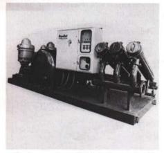
Custom-made prefabricated pumping stations are available from Aquaturf. The configuration of the pumps as well as the computer program for water distribution is customized for each user's needs. Each model is a complete pump station.
