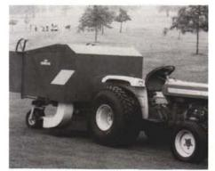
per can be hydraulically dumped by the operator without leaving his seat on the tractor. The vacuum can be converted quickly to blow debris up to 15 feet.
