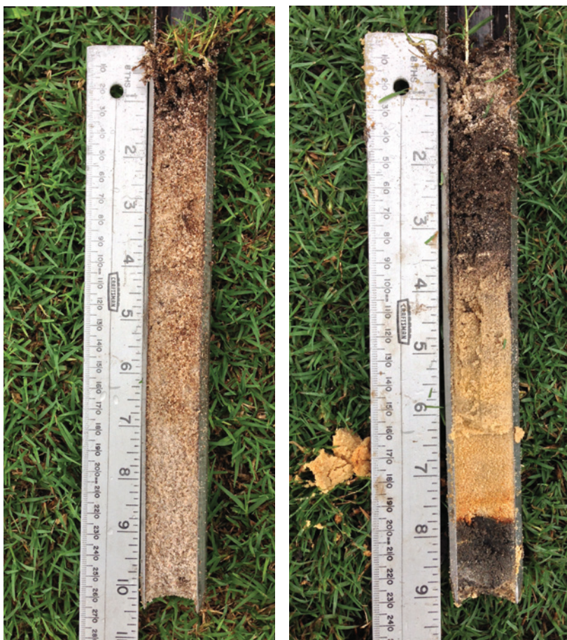
▲ Left (Photo 1) A soil core removed from an athletic field built with a sand-based rootzone. Note the consistent texture throughout the depth of the core, lack of any compacted layers and minimal organic matter accumulation at the surface.
