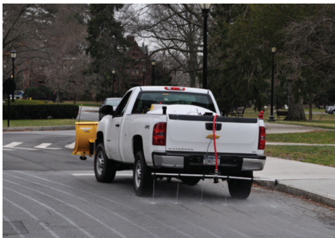
▲ Top: Storm water used for sports turf. Bottom: The grounds crew pre-treating campus roads with a salt brine.
