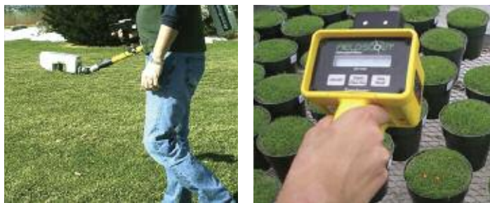
◀ Figure 4. Left: Greenseeker canopy reflectance sensor system. ▶ Figure 5. Right: Spectrum FieldScout chlorophyll meter.
