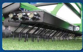
The spring tine rake attachment is equipment with 42 tines that comb through the turf surface, lifting fiber and infill, preparing the turf for exposure.
