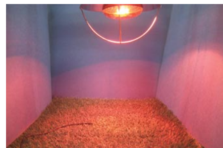
>> Figure 2. EXPERIMENTAL SETUP to evaluate surface temperature of synthetic turf.
