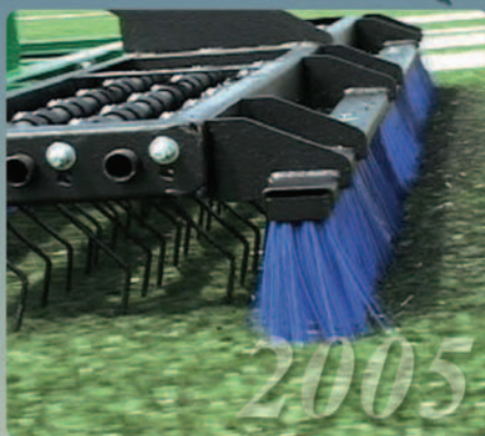
Spring Tine Rake Rear Brush Attachment
