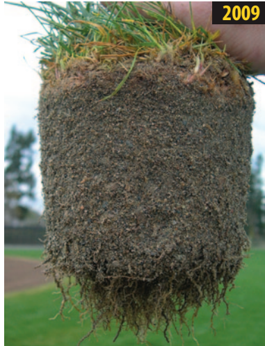
➤ Above: Redmond High School, Baseball & Softball Fields, Redmond, WA, designed by The Berger Partnership. Constructed with 10% CDE tilled into the top 6 inches of USGA sand and organic in 2002. 4 Years After Construction, 2006 7 Years After Construction, 2009
