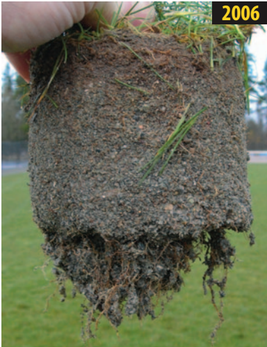
➤ Above: Redmond High School, Baseball & Softball Fields, Redmond, WA, designed by The Berger Partnership. Constructed with 10% CDE tilled into the top 6 inches of USGA sand and organic in 2002. 4 Years After Construction, 2006 7 Years After Construction, 2009
