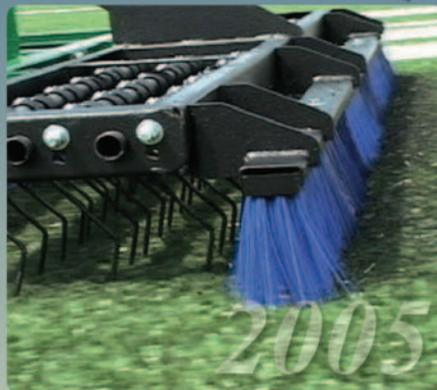
A valuable extension to the original Spring Tine Rake, the Rear Brush Attachment provides one-pass finish grooming and is fully adjustable to coincide with the brush wear on the Synthetic Sports Turf Groomer.
