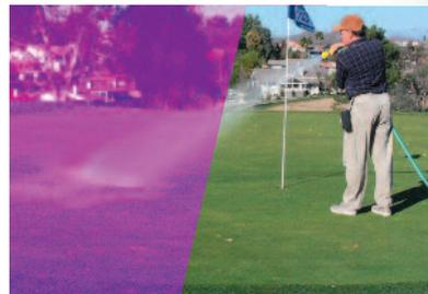
**HOW IT WORKS:** Dying vegetation absorbs and reflects sunlight differently than when it's healthy. The earliest signals occur at the outer limits of the human visual spectrum, and are rendered invisible compared to the predominant middle wavelengths. TurfSpy™ filters the light in the center so that fringe spectra, which show early plant stress, become visible.
