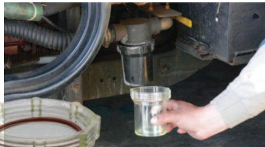
PelletPro's bowl, also sold individually, works perfectly as a replacement in-line filter bowl for most spray rigs. Heavy-duty, transparent plastic shows fluids. (No more cracked bowls during winter storage!)
