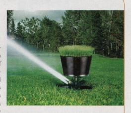
radius and an 8-in. pop-up height. The sod cup is 4-in. deep and holds a 9-in. wide section of natural grass. It is available as a valve-inhead or block model, and it virtually disappears when not in use. Can be used on synthetic turf. The part-circle heads are adjustable from 30° to 360° and can be switched into full-circle mode to syringe the infield and warning track areas.
