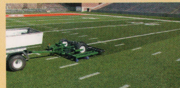
GreensSlicer Spring Tine Rake 3 rows of 28 tines.
