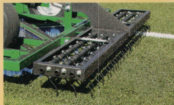
GreensSlicer Spring Tine Rake 3 rows of 28 tines.
