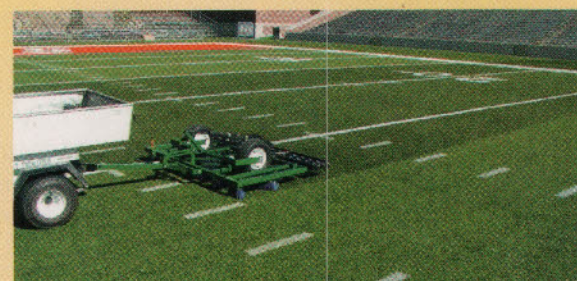
GreensSlicer Spring Tine Rake 3 rows of 28 tines.
