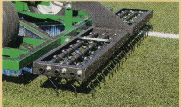
GreensSlicer Spring Tine Rake 3 rows of 28 tines.
