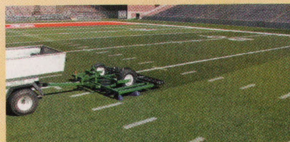
GreensSlicer Spring Tine Rake 3 rows of 28 tines.
