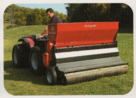
The OverSeeder's unequal disc slitting system actually plants the seed firmly in the ground. Boasting a tight spacing less than 3 inches, each seed coulter is individually suspended and accurately follows terrain. The new
