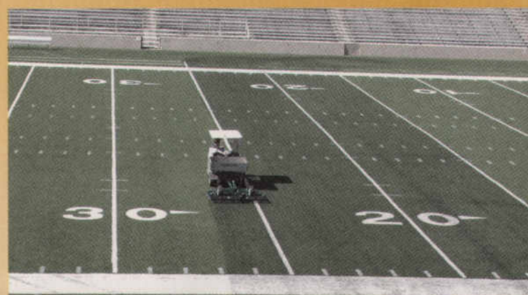
GreensSlicer Spring Tine Rake 3 rows of 28 tines.
