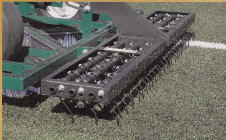
GreensSlicer Spring Tine Rake 3 rows of 28 tines.
