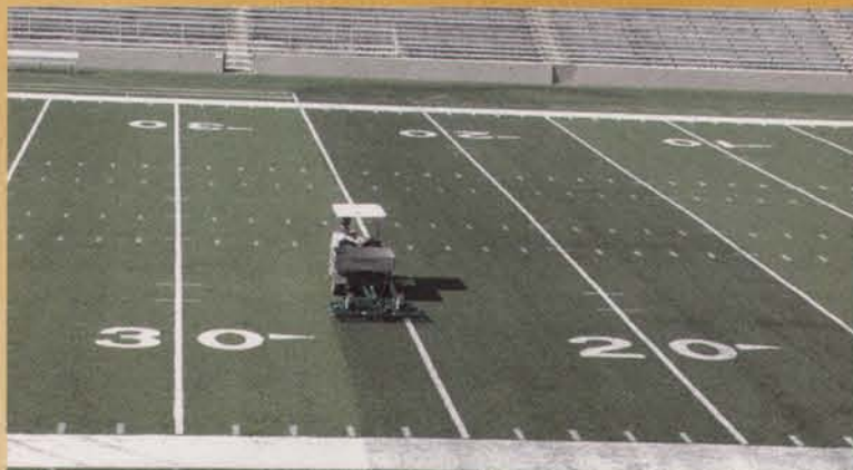
GreensSlicer Spring Tine Rake 3 rows of 28 tines.
