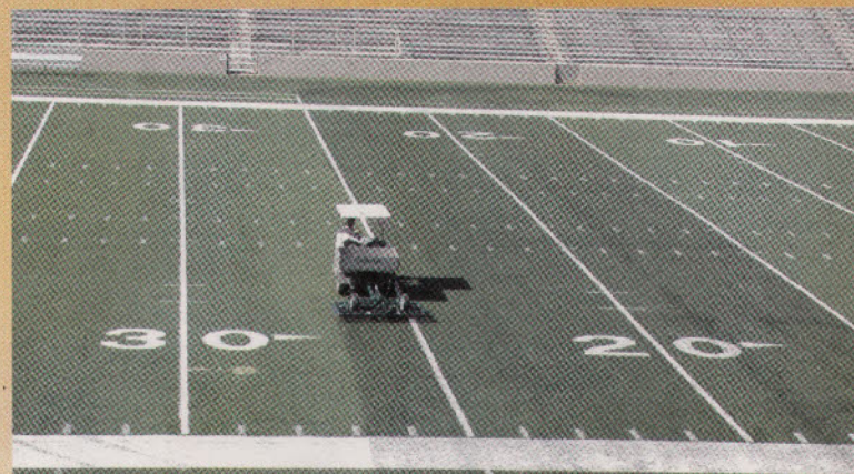
GreensSlicer Spring Tine Rake 3 rows of 28 tines.
