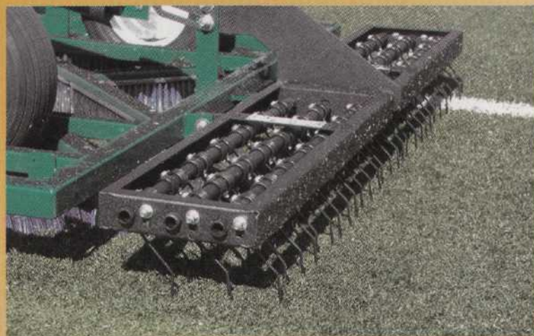
GreensSlicer Spring Tine Rake 3 rows of 28 tines.
