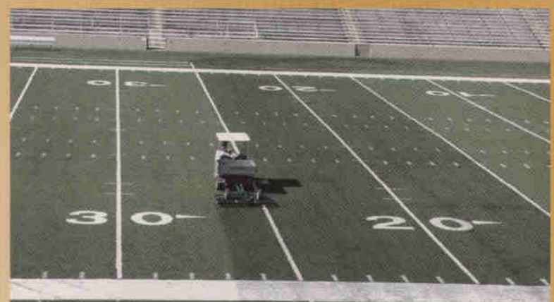
GreensSlicer Spring Tine Rake 3 rows of 28 tines.
