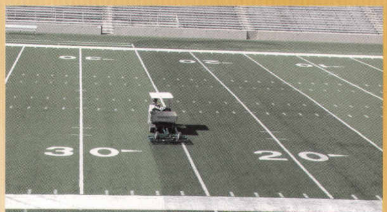
GreensSlicer Spring Tine Rake 3 rows of 28 tines.
