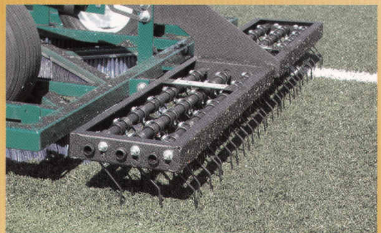
GreensSlicer Spring Tine Rake 3 rows of 28 tines.
