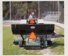
blades that are spaced 1-1/2 in. apart. The seed hopper has a capacity of 9.4 cu. ft. and will accept all seed varieties. Locke Turf/334-493-1300 For information, circle 175 or see http://www.oners.ims.ca/2909-175
