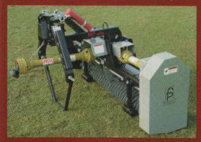
THE VC-60 IS DESIGNED FOR CONTINUOUS HEAVY DUTY OPERATION ON ALL TYPES OF SPORTS TURF. THE UNIT HAS A PATENTED SWING HITCH THAT ALLOWS THE OPERATOR TO VERTI-CUT AROUND OBJECTS WHILE TURNING, WITHOUT TEARING THE ESTABLISHED TURF. PIVOT POINTS DESIGNED ON THE HITCH ALLOW THE UNIT TO FLOAT OVER UNEVEN TERRAIN. THE VC-60 CUTTING DEPTH IS EASILY ADJUSTED IN THE FIELD, WITHOUT TOOLS "UP TO 11/2 INCHES DEEP" USING QUICK RELEASE PINS.
