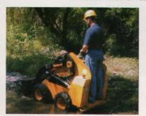
separate attachments. Machine is made to save labor on jobs such as small-scale dirt handling, utility installation, and lifting projects. Units have oil coolers and easy access to battery.
