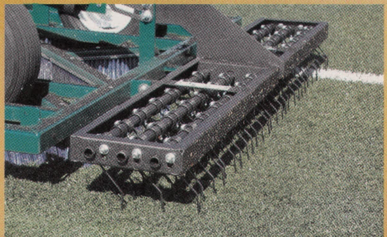
GreensSlicer Spring Tine Rake 3 rows of 28 tines.
