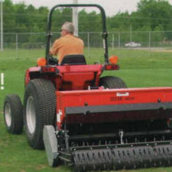
THE SE-60 SEEDA-VATOR IS THE ONLY SEEDER ON THE MARKET TODAY WITH THE FLEXIBILITY OF PRIMARY SEEDING OR OVERSEEDING WITH THE SAME MACHINE. THE UNIT HAS A PATENTED SWIVEL HITCH THAT ALLOWS THE OPERATOR TO TURN AROUND OBJECTS WITHOUT TEARING ESTABLISHED TURF. THE CLEATED ROLLER CAN BE PINNED TO GAGE TINE DEPTH. THE SE-60 USES PATENTED VIBRATING TINES TO FRACTURE THE SOIL, RESULTING IN AN IDEAL SEEDBED. THE SEEDA-VATOR COMES WITH EITHER GROUND DRIVEN OR ELECTRIC DRIVE SEED HOPPER.
