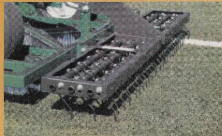
GreensSlicer Spring Tine Rake 3 rows of 28 tines.
