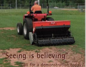
The First Products AERA-VATOR® uses a "patented" vibrating action to loosen and break up hard and compacted soils in the root zone, without destroying existing turf on the surface. The AERA-VATOR<sup>®</sup> has a unique swing hitch that allows the opera-tor to turn around objects without tearing the turf. The rear roller can be pinned to control tine depth up to 3 34 inches deep. The AERA-VATOR® comes in several models ranging from 40" to seeding or primary seeding.
