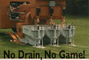
WaterWick's patented gravel-vein injection system creates a permanent answer to chronic wet turf problems. So the game goes on without delay.
