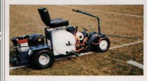
The Javdee Drive Liner is a self-propelled riding line marker. The 35-gallon paint tank carries enough marking material for a complete game field, or several practice fields. The 2-gallon flush tank cleans the discharge lines for work breaks, travel, or overnight. The center or side-mark spray shields are always operator-visible. A nearly zero turning radius reduces or eliminates back and turn maneuvers.
