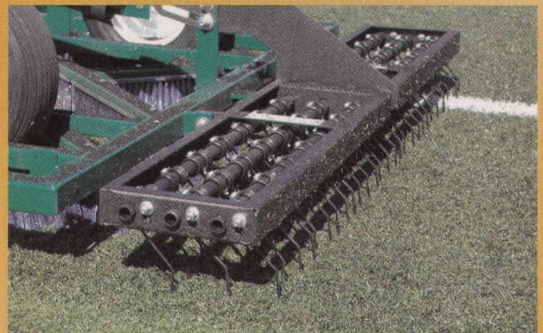
GreensSlicer Spring Tine Rake 3 rows of 28 tines.
