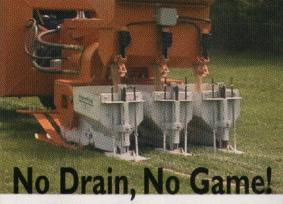
WaterWick's patented gravel-vein injection system creates a permanent answer to chronic wet turf problems. So the game goes on without delay.
