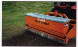
The SISIS TILTH N' SEED is a fast economical tractor drawn seeder with a wide range of seeding rates, down to 0.1oz. per sq. yard. The rakes create a good tilth and the rear roller firms the surface after seeding. The working width is  $64\frac{1}{2}$  in. - hopper capacity 7.8cu.ft.
