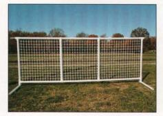
Signature Systems introduced a portable fence panel designed for athletic events, sport fields, and event venues. The panel is constructed from round versus square tube PVC. Instead of rigid pickets, the panel employs a plastic mesh, which is stretched in the fence frame. A rotating supporting leg system allows for compact and easy storage and installation and flexible foam enable panels to be connected to each other quickly. Signature Systems, LLC
