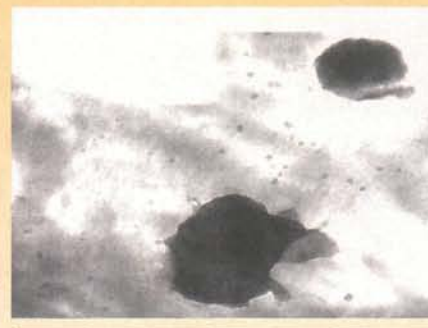
Figure 2. This TEM image shows the small colloidal nature of humates (less than two microns). The image depicts 45,000X magnification; the scale bar represents 0.1 microns. Courtesy: Michael DePew
