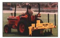
AerWay turf aerators give grounds managers more options for treating sports field compaction. A typical playing field can be
