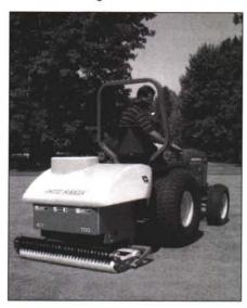
John Deere's RZI 700 Tractor Mounted Injection System:
