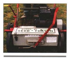
Although tractor-driven equipment is used on larger areas, this type of slitseeder can be used to cut grooves in the soil on targeted areas.
