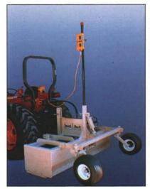
The Level Best laser-guided grading system can cut the time required to achieve finished grade by 300 percent or more, while maintaining a grading accuracy within 0.25inches. At a cost approximately 75 percent less than traditional grading equipment,
