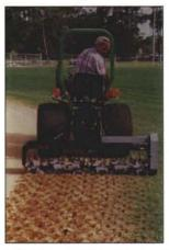
On grass sports fields aeration is possible without tearing the established turf. Guaranteed penetration in your hardest areas. (Play can resume immediately.) The AERA-VATOR\* provides excellent results by reconditioning skinned areas or mixing top dressing. Penetration is controlled by varying PTO & ground speed. (Total
