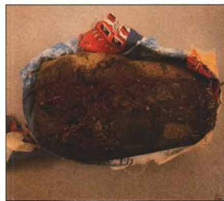
This soil core has been treated with a dipyrindyl indicator solution. The red staining on the core indicates the presence of reduced iron.
