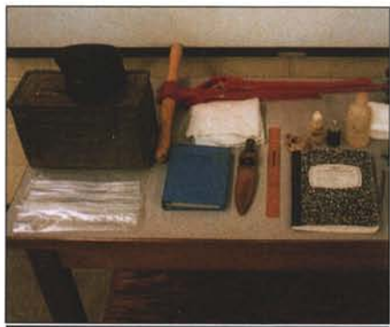
A field soil tool kit includes a cup cutter and a box large enough to hold a camera, color charts, thermometer, spray bottle, chemicals and other items. Photos courtesy: Michael DePew.
