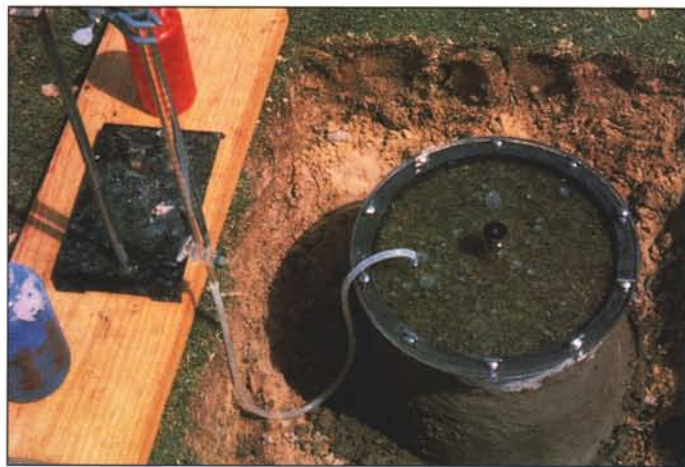
On-site readings of specific soil conditions are available through instruments such as Texas A & M's infiltrometer.
